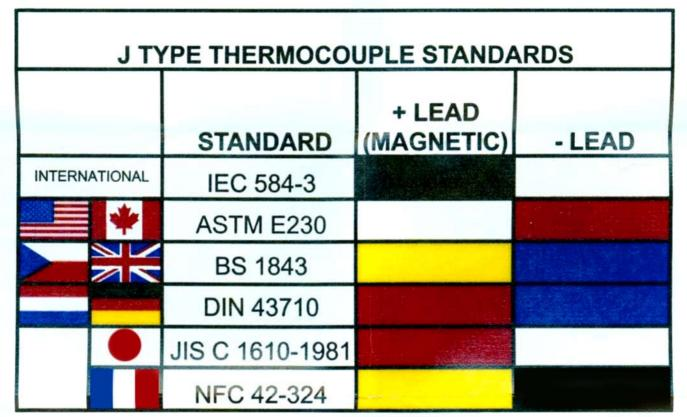
IF USING A DME HEATER WITH EMBEDDED THERMOCOUPLE AND THERMOCOUPLE WIRE COLORS ARE WHITE NEGATIVE (-) CONSTANTAN (NON-MAGNETIC) AND BLACK POSITIVE (+) IRON (MAGNETIC) HEATER POWER LEADS WILL BE MULTICOLOR.
