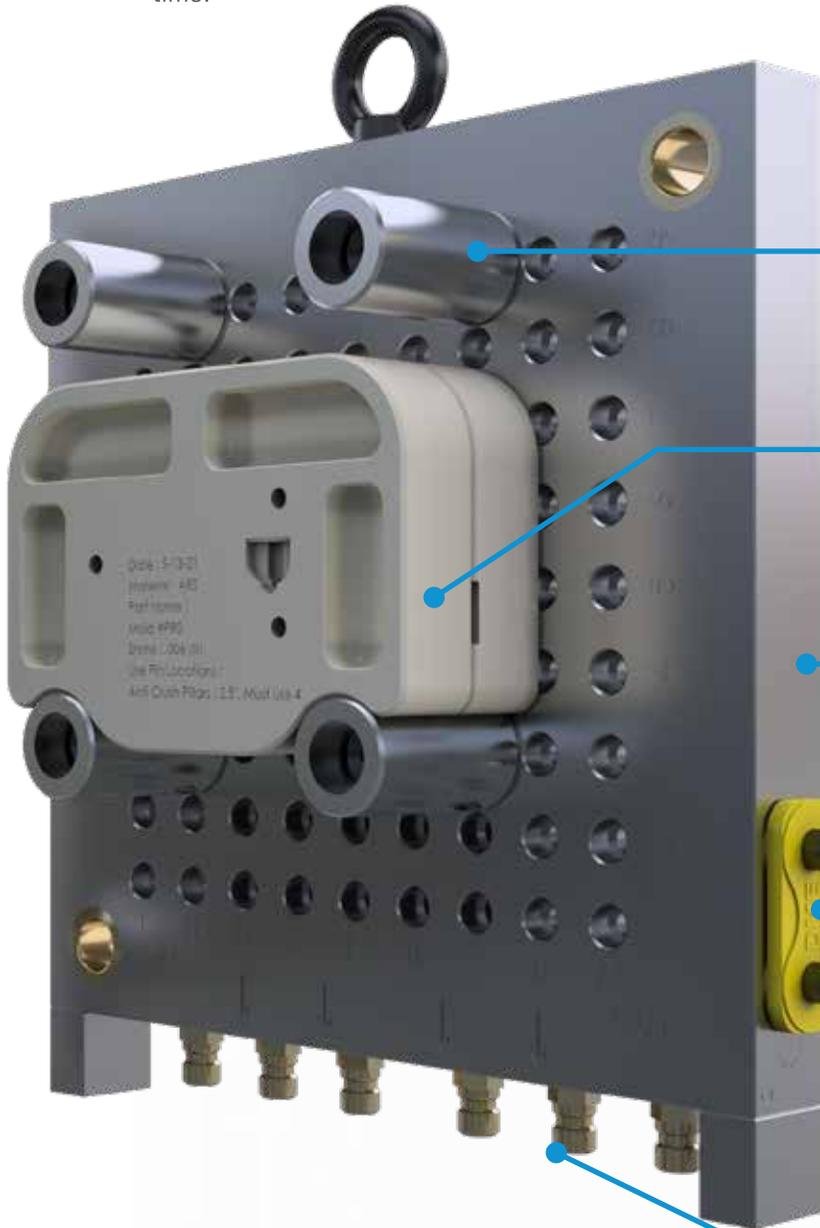
**Support Pillars** – 3/8" thread, Support Pillars ensure the cavity and core have the precise clamp force to prevent flashing of the part or any damage to the resin mold.
