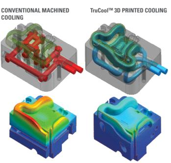
TruCool conformal cooling provides superior heat transfer over conventional cooling technologies.
